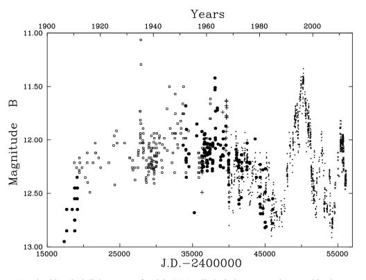
Figure 1: The historical light curve of NGC 4151. Filed circles – our photographic data, open circles – Pacholszyk et. al. (1983), pluses – photoelectric data obtained before 1968, dots – Crimean photoelectric monitoring, x – our new photoelectric and CCD data. The errors are of the order of 0.2 mag for Pachalcsyk's data, 0.1 mag or better for our photographic points, and ~ 0,02 mag for out photoelectric and CCD data.
