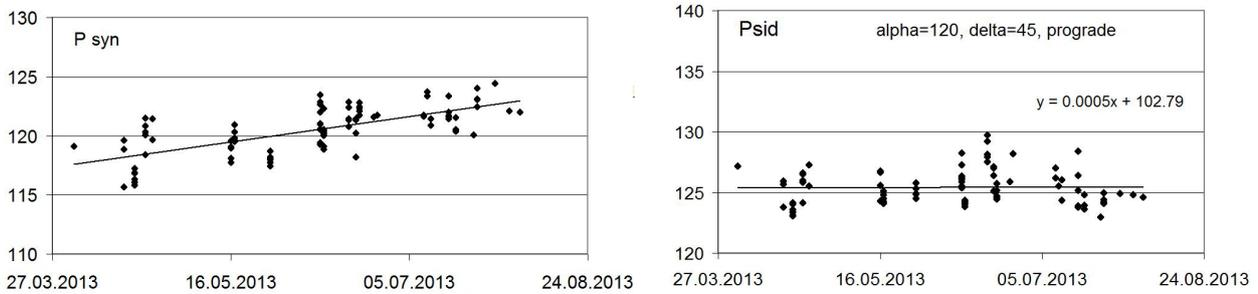
Figure 3: a) the measured values of the EnviSat space craft synodic rotation period; b) the optimal solution for the rotation pole ( $\alpha_p = 120^\circ$ ,  $\delta_p = 45^\circ$ , the prograde rotation), deduced by the method accounting for parallactic shift of flashes on the light curve. At that, the average sidereal rotation period within 4 months is almost constant and equals to 125.6 sec.
