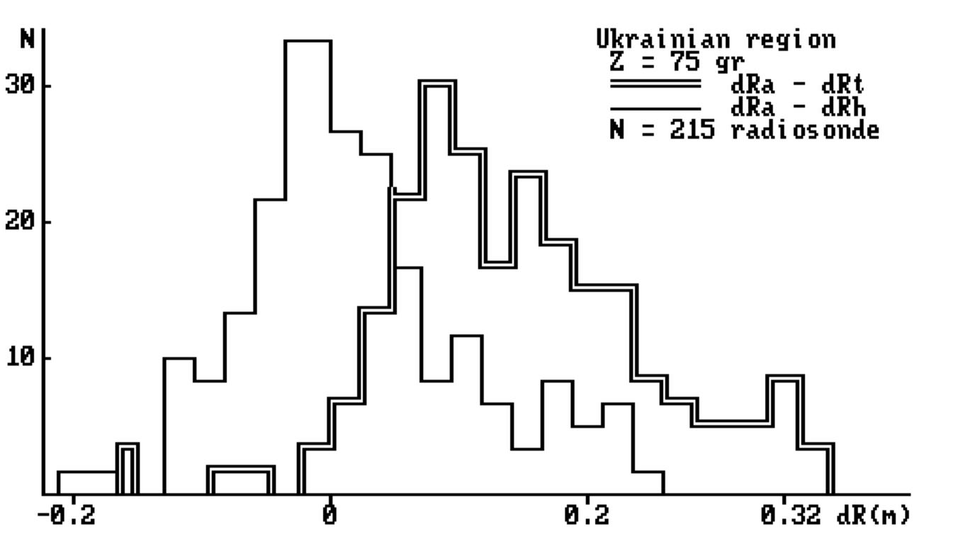
Figure 1: Figure 1. The histogram of the differences between the wet component tropospheric delay obtained according to the radiosonde data and the thermodynamic model (double line). The solid line - according to the radiosonde data and Hopfield's model.
